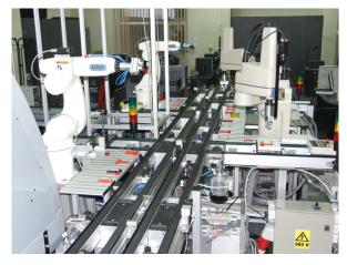
Fig. 6. Layout of the manufacturing cell with holonic control
