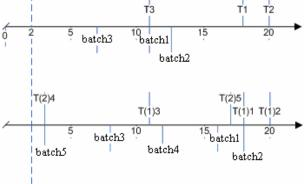
Fig .7. Inserting new batches among executing ones with the EDF algorithm.
