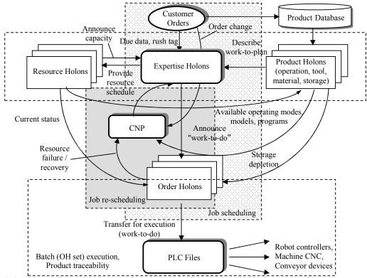
Fig. 2. Basic holon cooperation and communication structure in the semi-heterarchical control architecture
