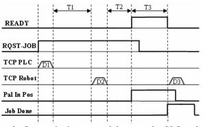
Fig. 3. Communication protocol between the PLC and a Robot Controller authorizing an OH operation execution
