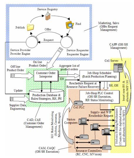
Fig. 1 - SOA integrates job-shop, team-based manufacturing with holonic robot control
