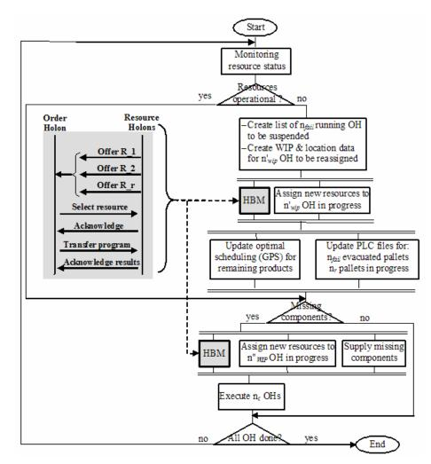
Fig.4. Dynamic OH rescheduling at resource failure/storage depletion with embedded CNP job negotiation (monex)
