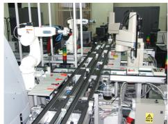
Fig. 5. Layout of the manufacturing cell with holonic control
