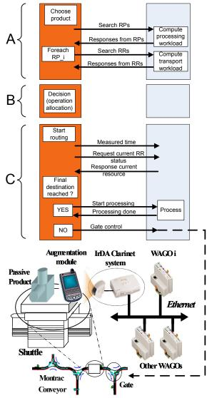
Figure 7 System architecture and order-resource interactions for routing and allocation
