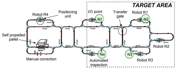
Figure 6 AIP cell system layout
