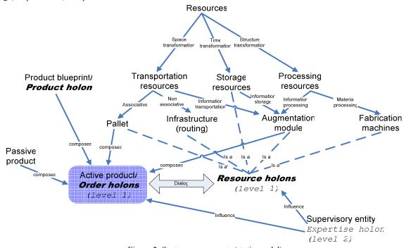
Figure 2 System components (static model)
