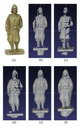
Fig. 5. Reconstruction of a decorative object (a) - photography; (b), (c), (d) - scans from different orientations; (e) - the scans merged into a single mesh; (f) - 3D surface model created using the Poisson filter in MeshLab.
