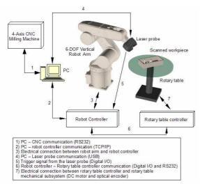
Fig. 1. Overview of the laser scanning system
