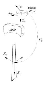
Fig. 2. Tool transformation for the laser probe.
