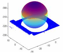
Fig. 3. Sphere identification and fitting from 3D point cloud data.
