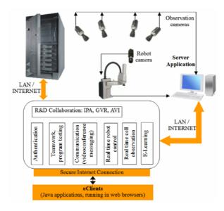
Fig. 1. The structure of the collaboration portal & communication platform
