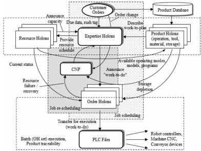
Fig. 1.3. Basic holon cooperation and communication structure in the semi-heterarchical control architecture
