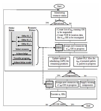
Fig.1.5. Dynamic OH rescheduling at resource failure/storage depletion with embedded CNP job negotiation (monex)
