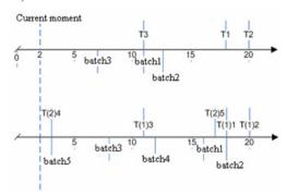
$Fig\ .\ 1.8.\ Inserting\ new\ batches\ among\ executing\ ones\ with\ the\ EDF\ algorithm.$
