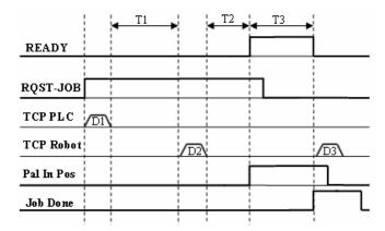
Fig. 1.4. Communication protocol between the PLC and a Robot Controller authorizing an OH operation execution
