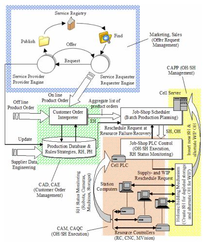
Fig. 1.1 – SOA integrates job-shop, team-based manufacturing with holonic robot control
