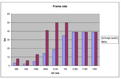
Fig. 19. FPS for external network, constant bit rate, priority: Image quality, fps
