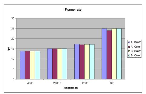
Fig. 13. FPS rate for MPEG-4 encoding
