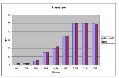
Fig. 17. FPS for internal network, variable bit rate, stream optimization: Bandwidth, fps
