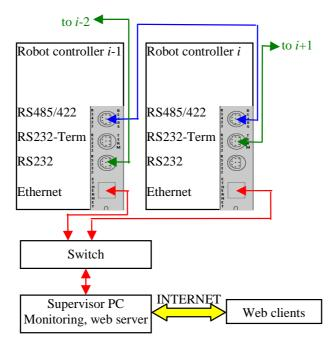
Fig. 23. Fault-tolerant communication architecture
