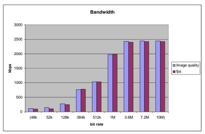
Fig. 16. Bandwidth for internal network, constant bit rate, priority: Image quality, fps
