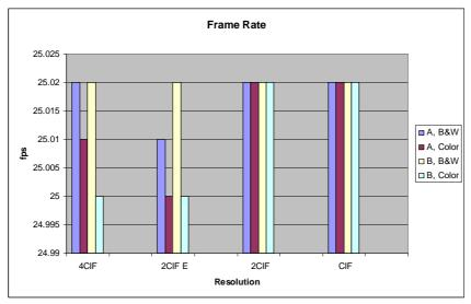
Fig. 11. FPS rate for Motion JPEG encoding
