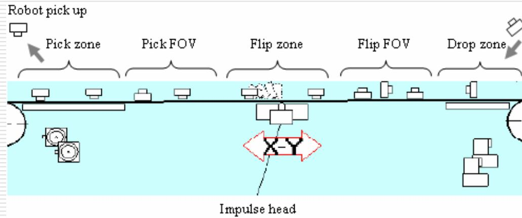
Fig. 13 – X-Y flipping mechanism
