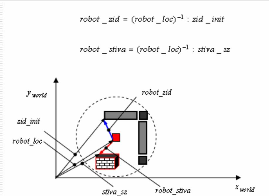
Fig. 5 – Computing the *relative transformations* to access respectively the base of the brick pallet and of the wall segment
