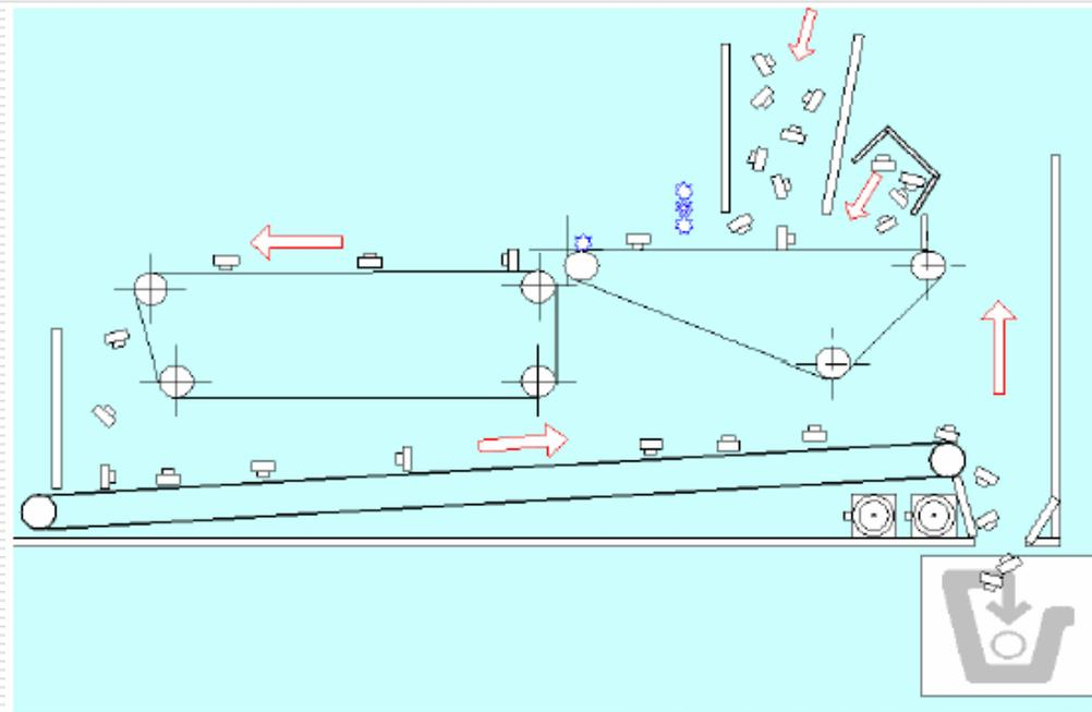
Fig. 12 – X-Y flipping mechanism
