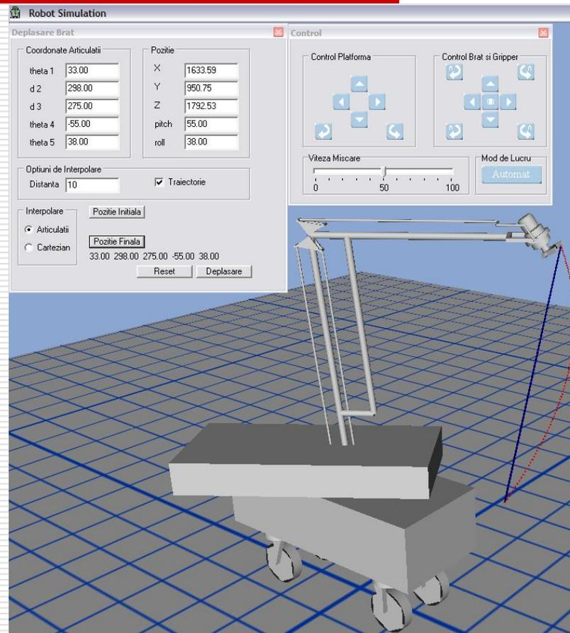
Fig.6 – Simulation results for RMRC and electronic gear path control of the robot arm
