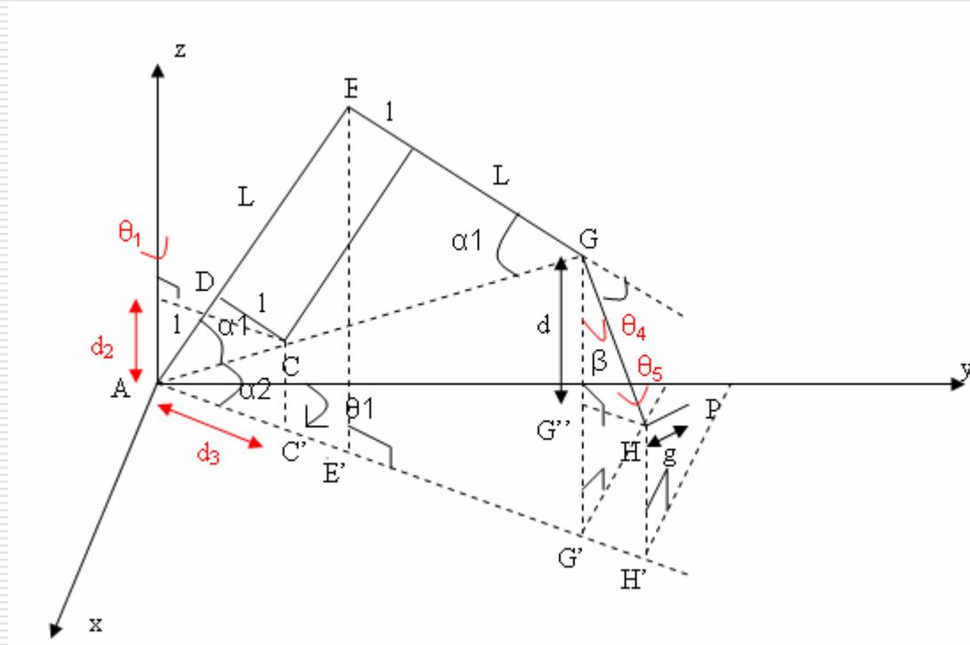
Fig. 2 – The close-chain kinematic structure 5-d.o.f. cylindrical robot manipulator.
