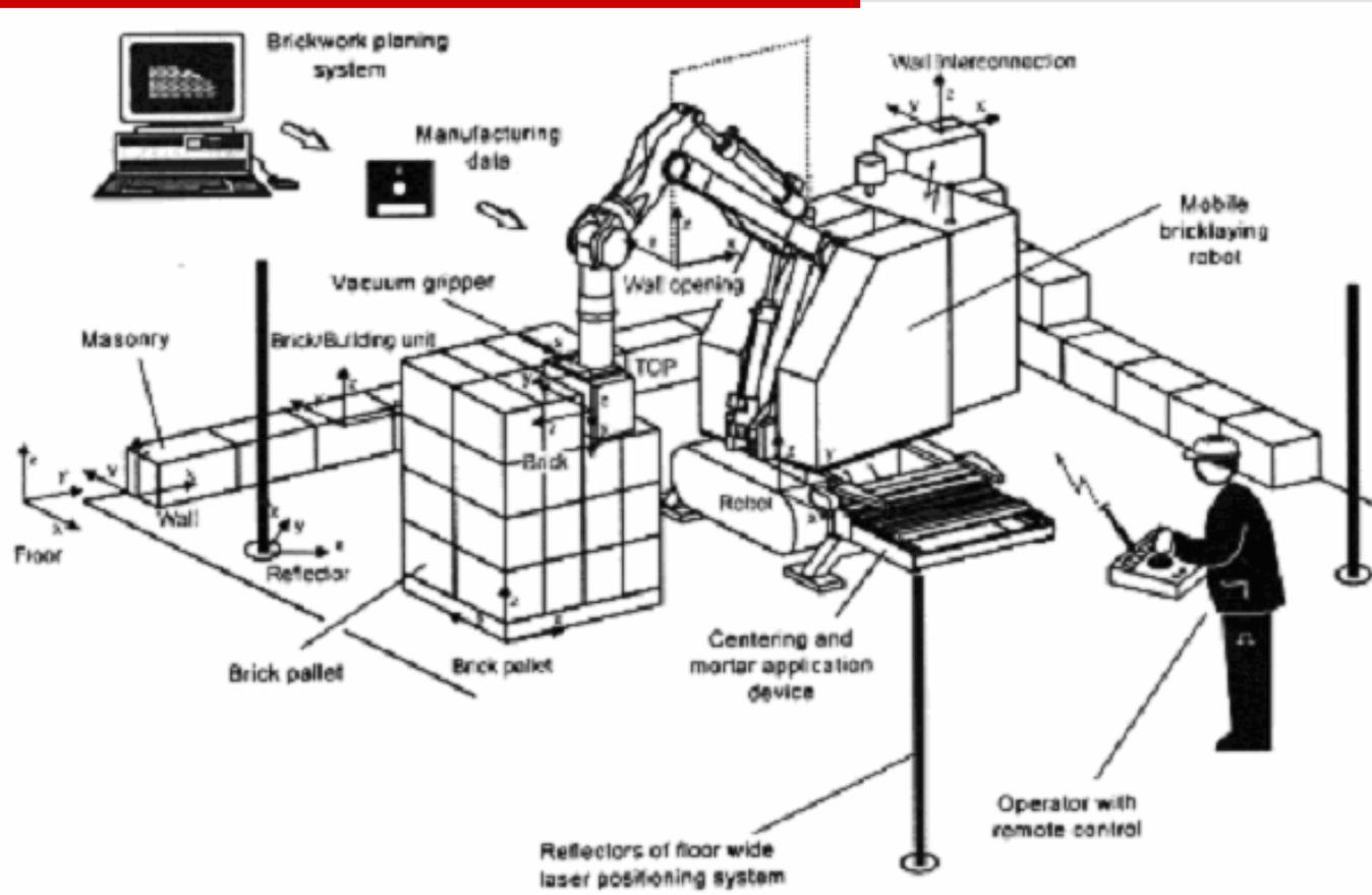
Fig. 1 – The 7-d.o.f. mobile construction robot and its working environment.
