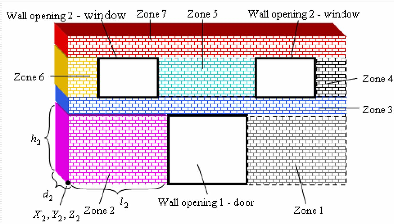
Fig. 3 – Stage 1: extraction of geometry data and locating data for elementary wall zones (from architecture plans and construction specs.)
