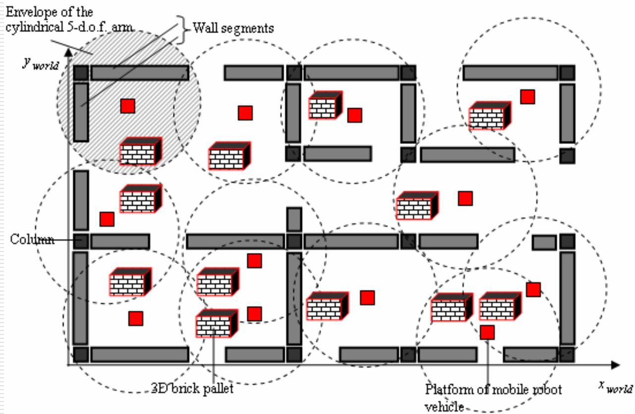
Fig. 4 – Partitioning a global masonry task in 12 bricklaying subtasks each one associated to a wall segment
