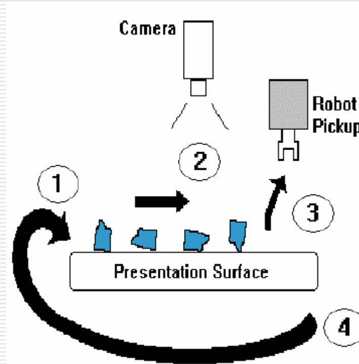
Fig. 9 – Basic flexible feeding concept: 1 – supply parts;
